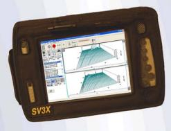
The SV3X's four (4) or eight (8) channel configuration and unmatched versatility makes finding and repairing machinery faults easy while saving you considerable time, money, and effort.
