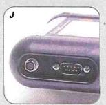
Countersunk connectors, well protected against external damage.
