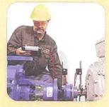
user you are given step-by-step instructions on the display through the entire measurement procedure. Even though the technology inside is rather advanced, the measurement principle is straightforward. It is based on the "reverse indicator method" with two laser/measuring units mounted on each side of the coupling.
