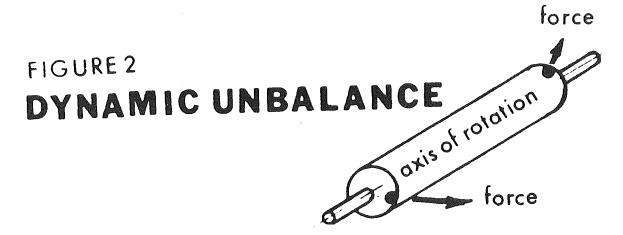
Static unbalance can usually be detected by using a conventional gravity type knife edge balancing method, while dynamic unbalance necessitates the use of special balance machines requiring special skills and experience to accomplish a satisfactory balance condition.
