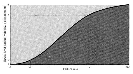
The SN curve: As peak velocity of vibrating elements goes up . . . the number of cycles to failure goes down
