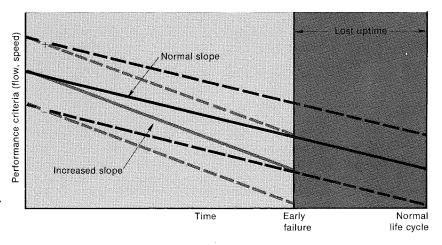
As stress levels increase . . . so does the failure rate
